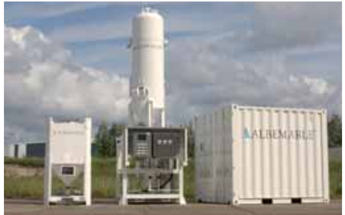
An AAU with a flow bin and a vacuum hopper.
